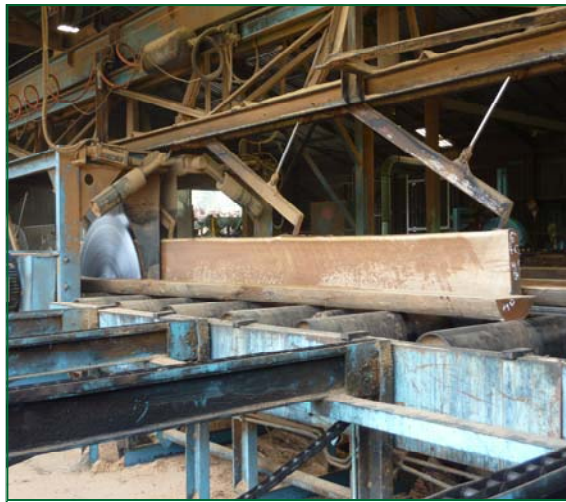
ABOVE LEFT: Saw trimming the log into slabs for docking. ABOVE RIGHT: Gordon Ford [Ford Timbers] and Gary McCarthy.
